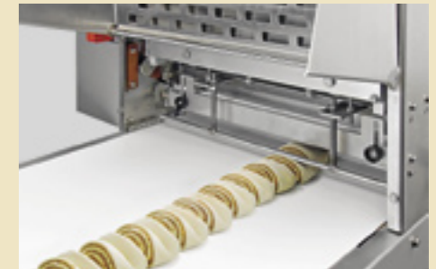
During cutting, the cinnamon (or raisin) rolls are embossed with a special stamping die.
