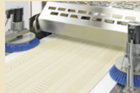
A large number of decorative rollers are available for double-folded pastries. You cut the patterns in the dough sheet before filling.
